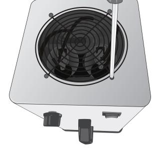
Gently remove the plastic end cap, screen and carbon filter.
